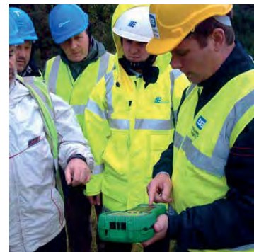
Measuring earthing resistance of the earth connection
