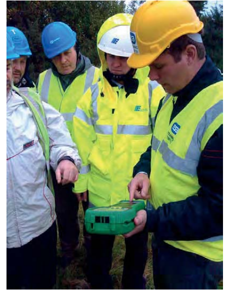
2. Measurement of ground resistance.
