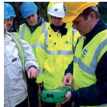
Measuring earthing resistance of the earth connection
