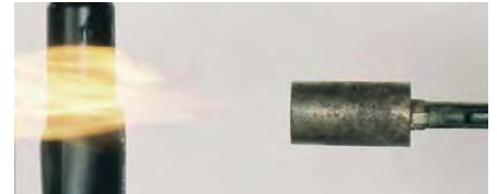
Shrinkage of the insulation is achieved by using heat.
