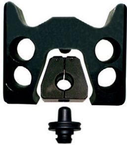
Matrix holder V2521, matrix P13M, punch P13D.
